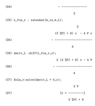
Since this is the only critical point found for L on the interval  $[0, P(\pi+2)^{-1}]$  this must give the absolute maximum for L. Maxima can now be instructed to find the ratio of r to h:
